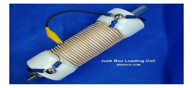
Junk-Box Loading Coil for QRP Antenna 40M > 10M
