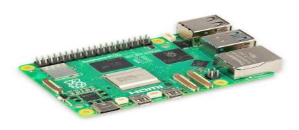
processor running at 2.4GHz, Raspberry Pi
